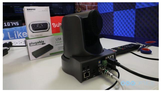
**Step 12** - Now that we have control of our cameras with our joystick controller it is time to set some PTZ presets. To do so, we can drive the camera(s) to specific positions of interest and once we have the camera at a PTZ preset location that we will want to recall in the future simply click the set button and the number you would like to save this position as and press enter. We can repeat this process with over 200 presets until we have saved every location that we desire.
