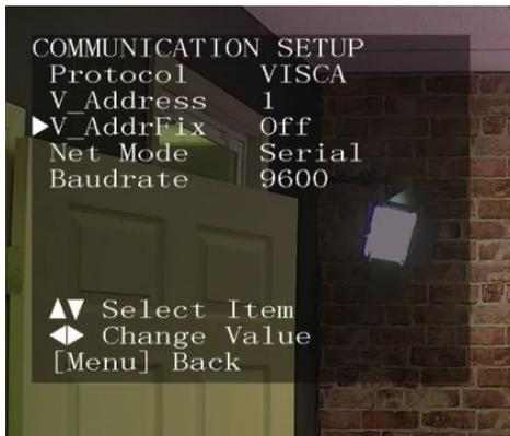
**Step 11** - Now let's verify that your first camera is set up properly. Bring up the OSD of the first camera and go to "setup" you can view the OSD menu on your video feed coming in to your computer via SDI. Make sure that the protocol is set to "VISCA", the Net Mode is "Serial", the V-AddrFix is "On", and the Baud Rate is "9600". Make sure the V\_Address is set to "1". You will need to repeat this process for each camera in your chain of control, setting each visca address to be unique.
