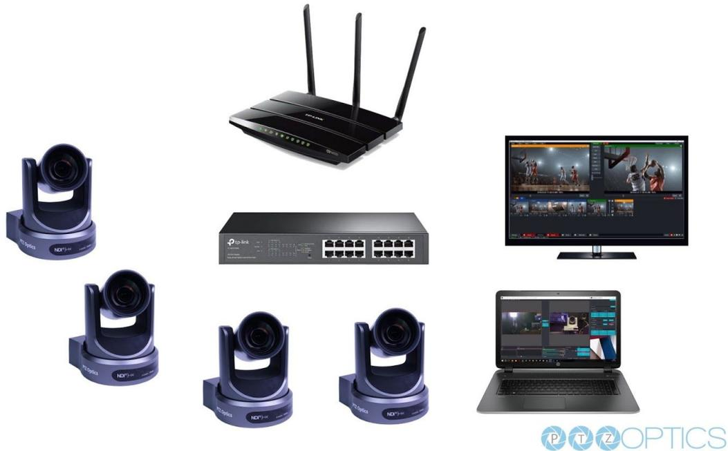
**Note:** Make sure that your network is setup to handle multicast traffic before enabling this feature. To use multicast each PTZOptics camera should have a unique multicast address. You can assign a multicast address in the “network” area of your cameras IP interface. Once you have determined a unique multicast address for the camera you can turn multicast on. You can turn multicast on by clicking the on radios button and clicking the apply button. Finally, reboot your camera.
