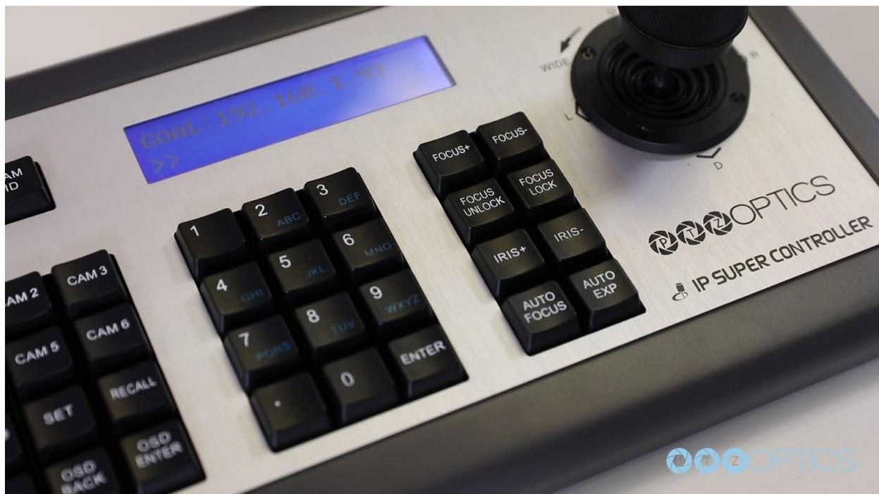
**Step 5** - The joystick is now ready to add cameras IP addresses. The SET UP button opens a menu on the LCD screen. Press the “ENTER” button to add a camera on setting “01/05” or “Add Camera”. Set a Device ID for the corresponding camera or Input the camera’s IP address into the joystick including the “.” between octets. Example: IP = 192.168.100.88
