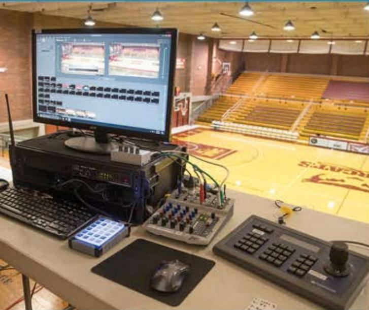
Here you can see the an example table setup for live streaming the action equip with a joystick controller and live streaming computer.
