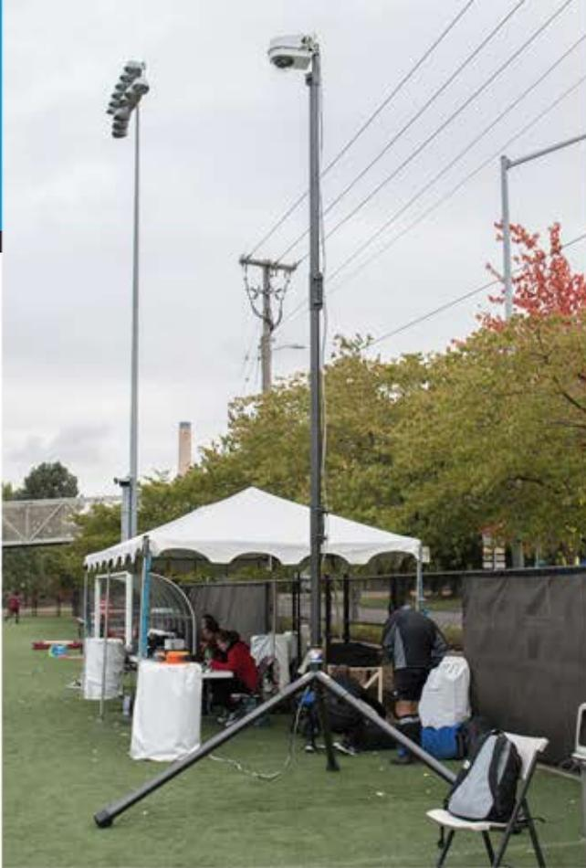
"I don't have a big production crew. So everything has been designed to be operated by myself or one other work study student" says Sabato. The Dotworkz outdoor camera enclosure is designed for permanent outdoor use and includes two weather sealed cable ports which Sabato uses for HD-SDI video and RJ45 converted to DB9 to be used for camera control with the HuddleCamHD joystick.
